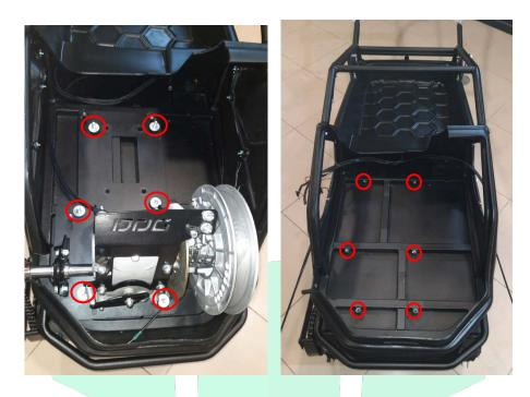
7. Extract the underframe with the reverse gearbox from the engine compartment and put them on the table for further locksmith works.
