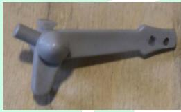
18. Return the air choke control lever at the original place.
