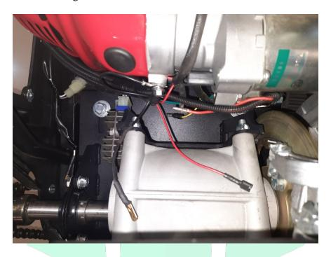
40. Connect wires to the accumulation battery terminals by the given way: the red wire in the corrugation to the «+» terminal. Connect the blue wire in the corrugation to the «-» terminal.
