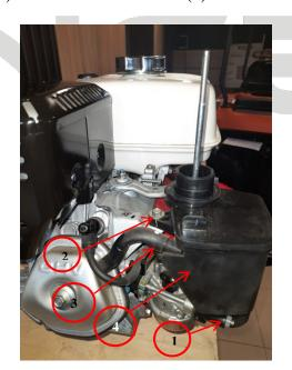
16. Weaken the throttle control lever that way, it will easy return back to the original position.
