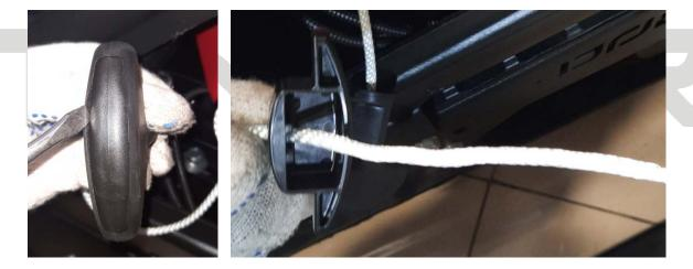
44. Pass the cable through the aperture in the right side cap, and then into the starter handle. Tie the knot and hide it in the handle.
