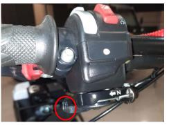
4. Apply power to the engine – move apply power switcher on the handlebar switch to the lower position.
