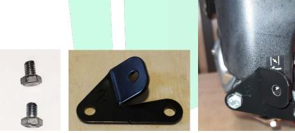
22. Take the spring fixation plate from the «Spring retainer kit» package № 3. Unscrew the two top bolts, that fixing manual starter cap and weaken the bottom bolt. Install the plate behind the manual starter cap. Look after the left bottom edge of the plate will not out of the manual starter cap. Screw the bolts.
