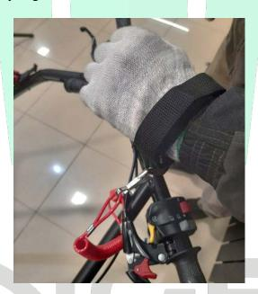
6. Start the engine: press on the yellow trigger of electrical starter.
