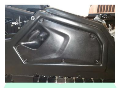
47. Anchor the left side cap, using screws with inner hex. Set the screw at the central bottom aperture, this screw is shorter than other 10 mm screws.
