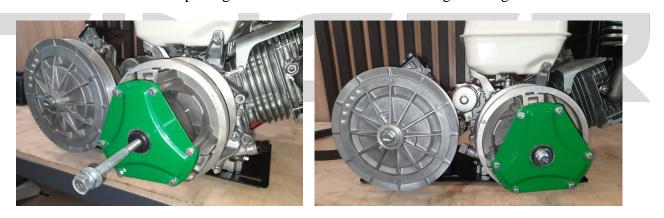
26. Take the CVT belt out of the box and dress it on the CVT. Tightening the belt and rotating the movable disc opposite the clock arrow movement, install the belt on the discs.
