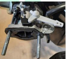
19. Install the manifold at the original place, anchor it by bolt. Connect the hose.
