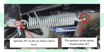
36. Turn the control throttle choke lever on the handbrake switch to the right (in "OFF" position). Install tensioner bolt in throttle choke cable plate  $N \ge 2$ . Pass the choke cable through the tensioner cable (1), then through the aperture  $N \ge 2$  at the lever (2) and then fix the end of the cable by the  $\emptyset$  3 mm cable fixator (3).
