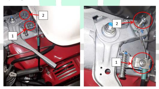
34. Take the M7 cable tensioner bolt and 3mm cable fixator and Ø14 mm spring out of the «Spirings and retainers kit» package №6. Connect the throttle choke cable with yellow braid.
