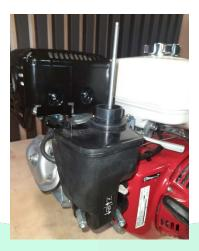
21. Take the two M6x10 DIN 933 bolts from the «Fasteners kit» package Nel 1 out. Take the plate of throttle choke cable out of the «Remote choke kit» package Nel 2. Install the plate on the M6 sleevenuts with the two M6x10 DN933 bolts.
