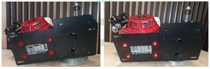
13. In presence of plastic cover attached to the bottom part of the engine and air filter, demount it.
