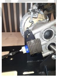
24. Prepare the engine shaft for CVT installation. There is a key in shaft's groove. Take the Safari CVT out from the box. Aligning the CVT groove with shaft groove and holding the key, install the CVT on the shaft till stop.
