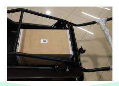
2. Detach bonnet rubber fasteners from the bosses on the frame at the left and right sides. Demount the bonnet.
