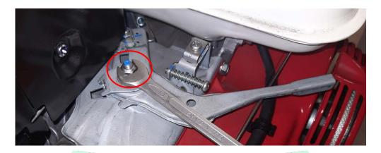
17. Demount the air choke control lever. Drill two holes on the lever:  $1^{st}$  one from the lever's edge to the center of aperture 5mm,  $2^{nd}$  one from the lever's edge to the center of aperture 10mm. Use the  $\emptyset$  2 drill bit.
