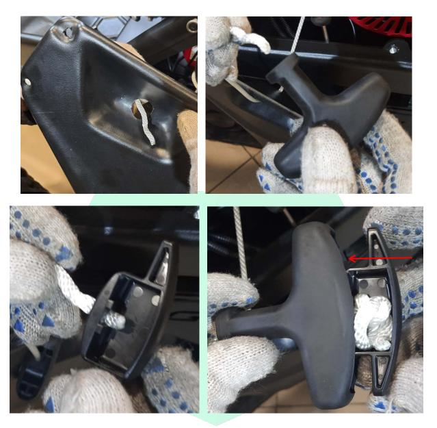
45. Take the tool out of the loop and untie the loop. Holding the side cap and handle, return the cable back to the place.
