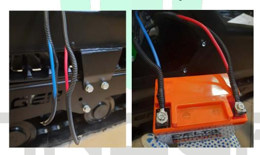
41. Install the accumulation battery at the engine compartment behind the CVT. Take the accumulation battery fastener belt out of the package  $Noldsymbol{0}$ 7. Anchor the fastener belt with a tongue to the hook behind the accumulation battery. Anchor the belt hook at the front of the battery to the hook by tightening the the belt tongue.
