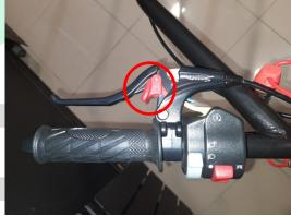
3. Open the throttle valve- turn the control choke handle to the left.
