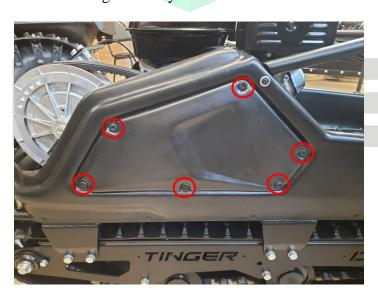
6. Unscrew the bolts that are anchoring the underframe with the reverse gearbox to the frame.
