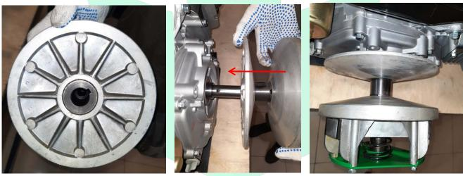
25. Take the 12x110 7/16"-20 UNF bolt, the M12 DIN 125 washer and the M12 DIN 127 engraved washer out of «Fasteners kit» package №1. Anchor the CVT on the engine using listed fasteners.
