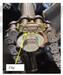
31. Moving the underframe backward to the movement way, regulate the chain tension. A normally tightened chain will have a sag of 10-20 mm at the middle between the sprockets. The sag is less than 5mm affects to the faster chain stretch, as result- fast sprockets worn out. Too stretched chain might fly down from the sprockets during the run. Slack chain should be tightened.
