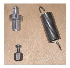
35. Anchor the one end of the  $\emptyset$ 14 mm spring to the aperture in sping fixation plate  $\mathbb{N}_{2}$ 3, the opposite end to the aperture  $\mathbb{N}_{2}$ 1 at the air choke control lever.
