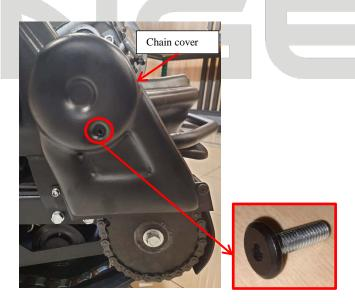
4. Take the chain out from the reverse gearbox sprocket. For that, demount the clip from the lock, then dismantle the opposite lock part and take the lock out of chain links.
