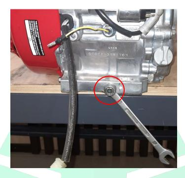
10. Unscrew the oil filler plug, pour required volume of oil according to the instruction, that is attached to the engine. Twist oil filler plug on.
